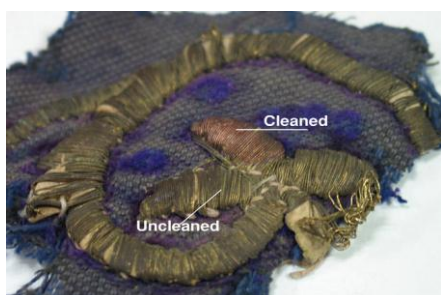
Fig. 5: An optical microscopy image shows the surface appearance of the metal threads after laser cleaning [21].
