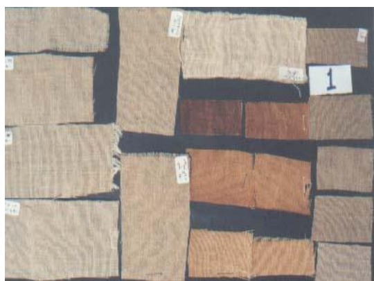
Fig. 7: The effect of a variety of tested polymers on linen textile after ageing by light for 200 hours, some of these polymers reduced the deterioration of the textile while others caused the textile to become stiffer and dry with browned colors.
