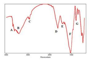
Fig. 7. FTIR spectrum of mud brick samples from Roman bath in Karanis.
