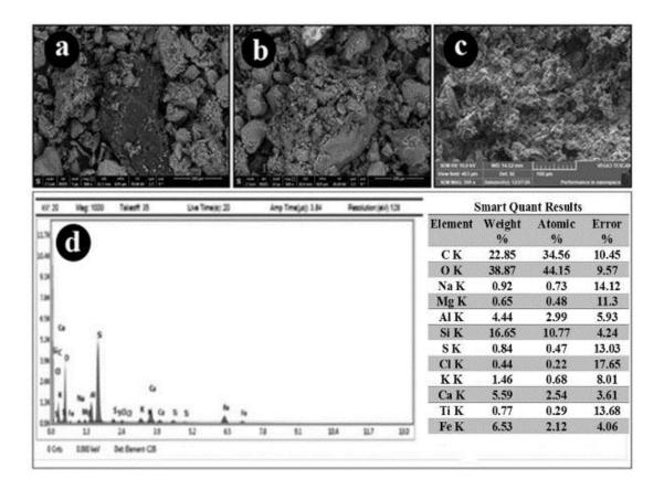
Fig. 9. SEM-EDX results of studied samples (a) SEM photomicrograph of mud brick, (b) SEM photomicrograph of mud mortar, (c) SEM photomicrograph of fired brick, (d) Energy dispersive X-ray (EDX) spot analysis of mud brick samples
