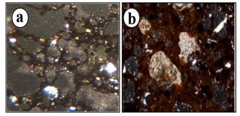
Fig. 8. PLM photomicrographs of studied fired brick samples (a) Showing quartz in rounded shape of very fine to fine-grained size, in addition to clay minerals and carbonate as cement materials, moreover iron oxides, pores and cavities are shown (25 X, CN.), (b) Showing quartz in rounded to angular shape, iron oxides, concretions of carbonates or clays floating in the clay cement, fragments and mafic minerals (10 X, CN.)
