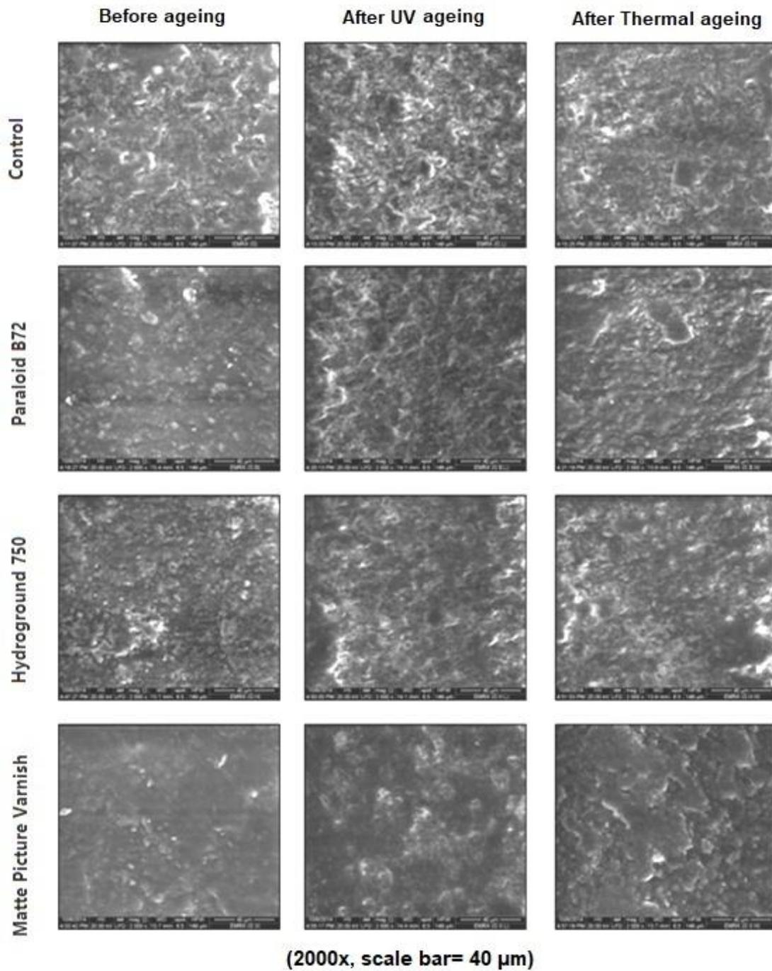
Fig. 7. FE-SEM micrographs (2000x, scale bar = 40μm) of the treated green painted samples before and after UV/thermal ageing
