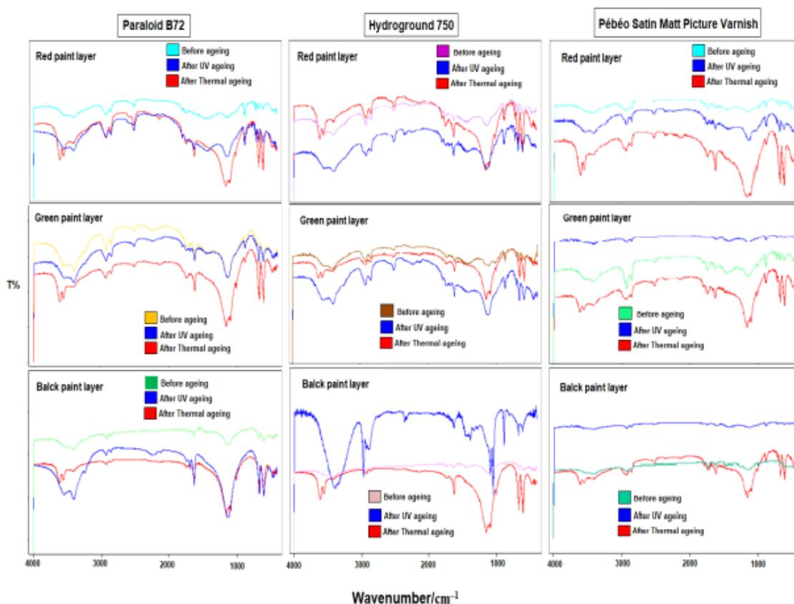
**Fig. 9.** FTIR spectra recorded on the treated laboratory models, before and after UV/thermal ageing
