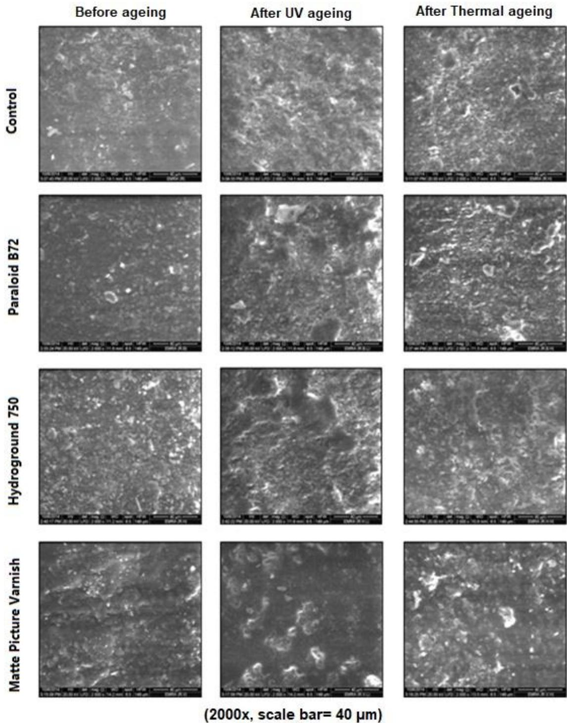
Fig. 6. FE-SEM micrographs (2000x, scale bar = 40μm) of the treated red painted samples before and after UV/thermal ageing.
