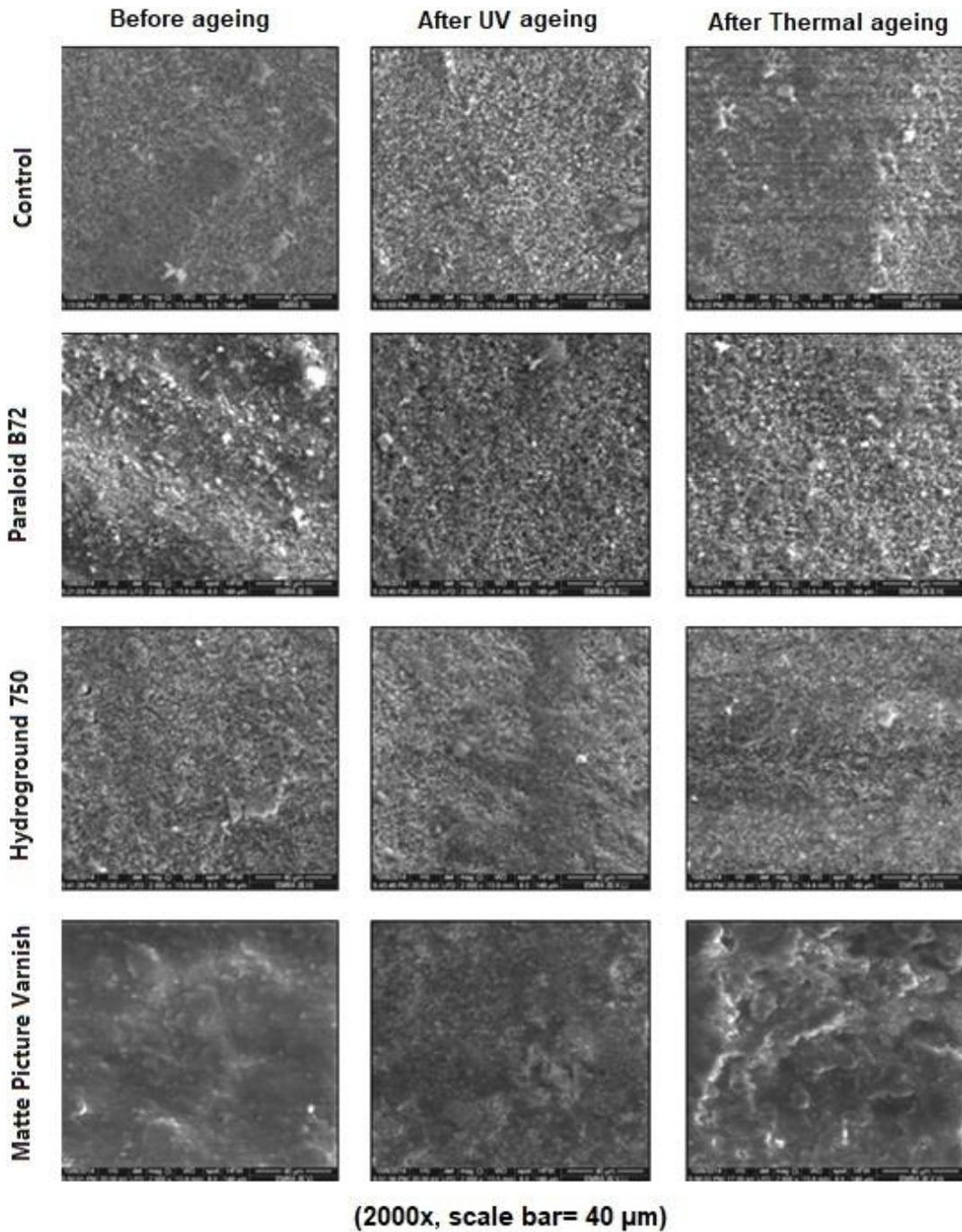
Fig. 8. FE-SEM micrographs (2000x, scale bar = 40μm) of the treated black painted samples before and after UV/thermal ageing.
