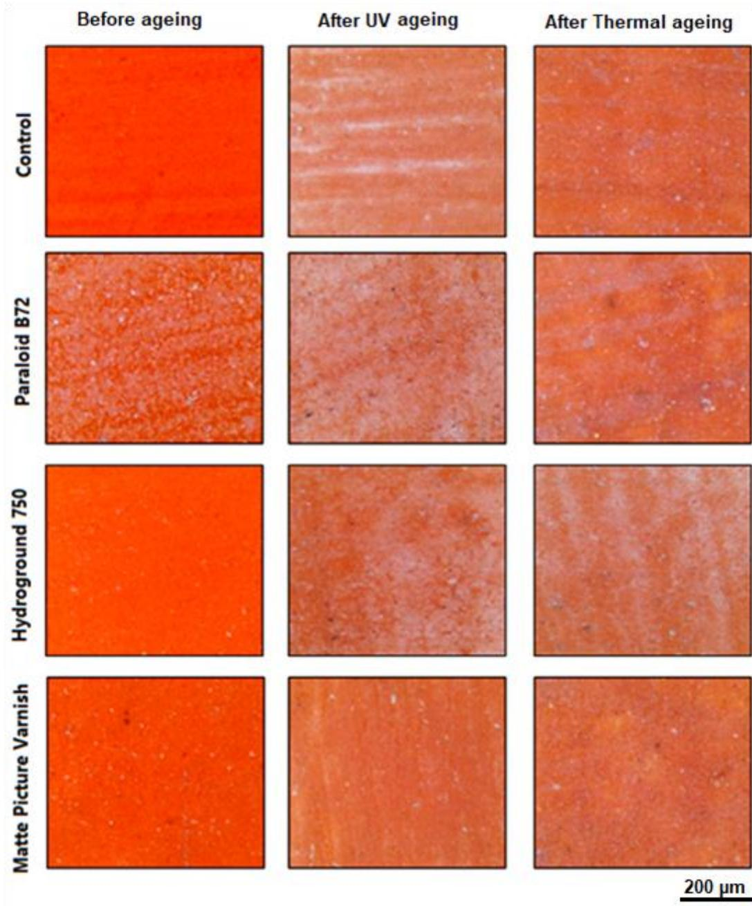
Fig. 2. Microscopic images (at magnification 100 X, scale bar=200 $\mu$ m) of the appearance of red painted models before and after UV/thermal ageing.
