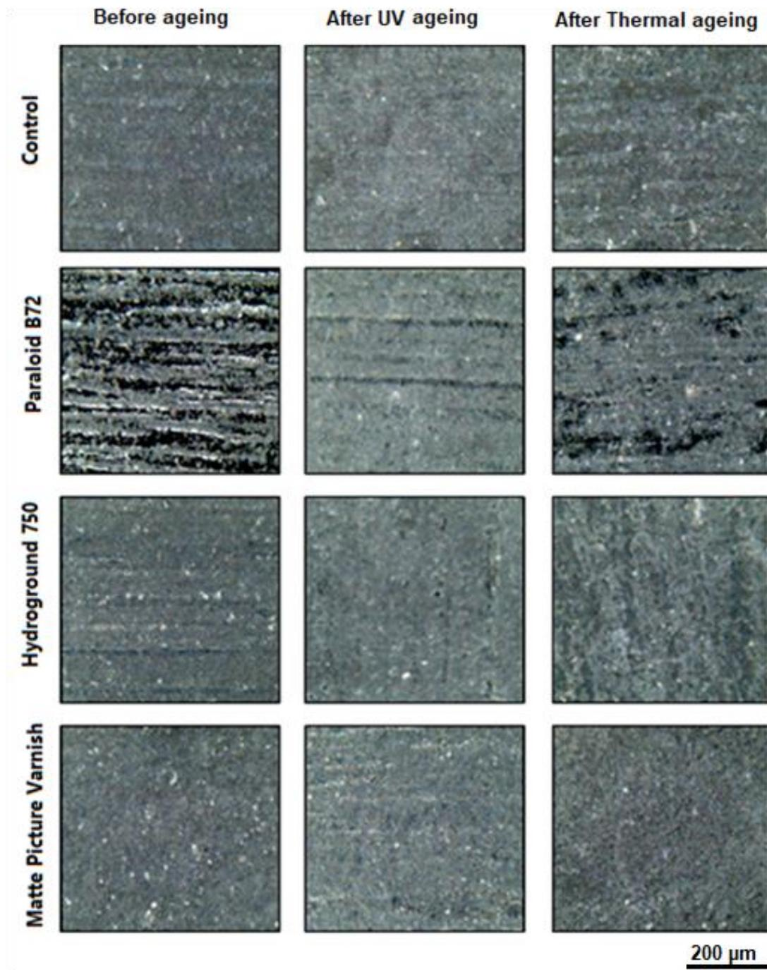
Fig. 4. Microscopic images show (at magnification 100 X, scale bar=200 $\mu$ m) the appearance of black painted models before and after UV/thermal ageing.
