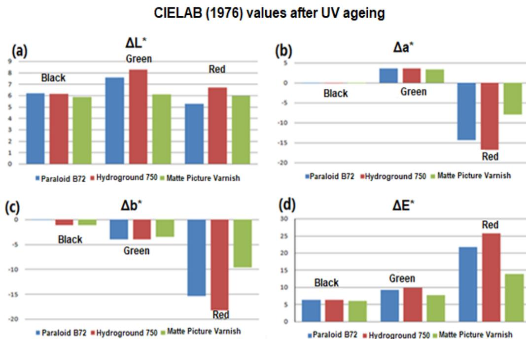
**Fig. 5.**  $\Delta L^*$ ,  $\Delta a^*$ ,  $\Delta b^*$  chromatic values and colour difference ( $\Delta E^*$ ) after UV ageing of the laboratory painted models.
