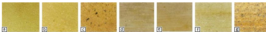
Fig. 1. Comparison between samples (a) bees wax before exposure, (b) bees wax after indirect sunlight exposure, (c) bees wax after direct sunlight exposure. (d) untreated wood, (e) wood after bees wax application, (f) bees wax treated wood after indirect sunlight exposure, (g) bees wax treated wood after direct sunlight exposure.
