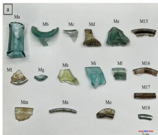
Fig.1: Decolorized and nearly colorless glasses from Roman period [3]
