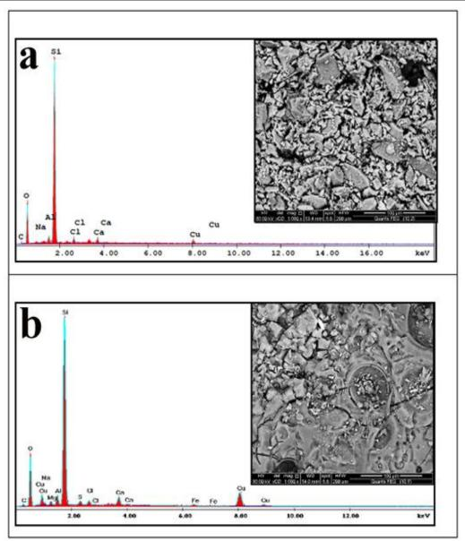
Fig. 8. Shows SEM/EDX results of the faience, a. The core, b. The glaze layer
