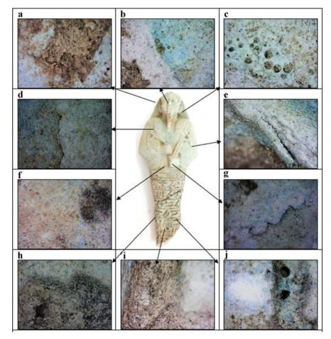
Fig. 5. Shows the examination by USB digital light microscope (the front), a. Dirt and dust penetrating the surface, b. Loss of glaze, c. holes in the glaze layer (manufacturing defects), d. Micro-cracks, e.Glaze flaking, f. Black stains in the glaze, g. Detaching and peeling of glaze layer, h and i.Dust and sand inside the hieroglyph's letters, j. Big holes with dirt
