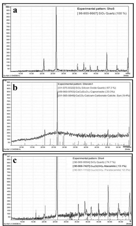
**Fig. 7.** XRD patterns of faience samples, a. Pattern of the core, b. Pattern of the glaze color, c. Pattern of the glaze discoloration
